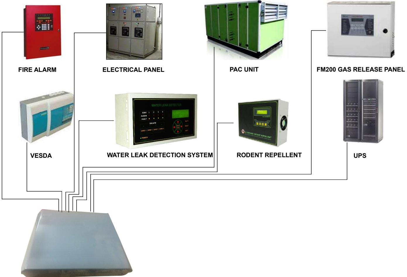
Server Room Critical parameters / Environment Monitoring System is complete solution including hardware and software bundled together. The Digital controller accepts 16 volt free digital inputs from various subsystems like FAS, Electrical, PAC, Gas Release, Vesda, WLD, URRS, UPS, Sprinkler etc.
