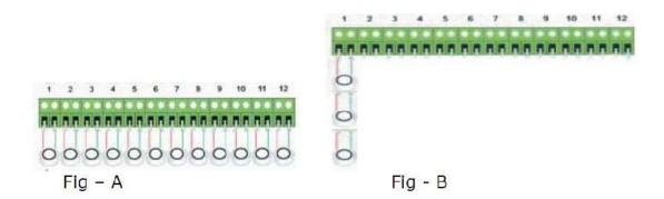
Connection details between C Systems URRS control panel and transducers. Fig A & B shows the possible wiring methods between transducers and Panel.
