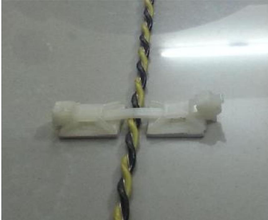
Use cable tie mounts and affix two such tie mount on either side of sensor cable as shown in figure. provide about 20 mm of space between two tie mounts in such a way that water shall pass through.
