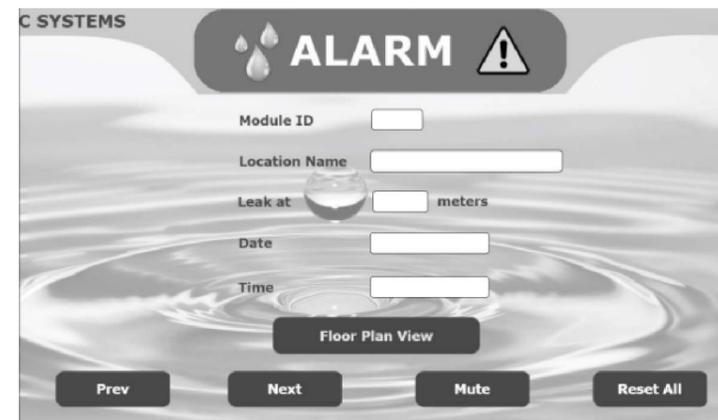
**Note:** Before pressing **Reset All** key, Ensure that leak origin & source are identified, rectified & sensor cables are cleaned with dry cotton cloth. Ensure the sensor cable is completely dry at any part otherwise, continuous alarms will be generated.
