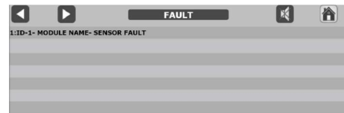
When **Fault** key is pressed in the main menu, the Fault list report screen appears as shown.
